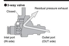
The 3-way valve can exhaust residual pressure (residual pressure remained in installed equipment) left behind in the outlet port side when air has been shut off.
