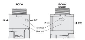
6. Do not place any weight of the product's piping or apply excessive torque on the product. When tightening the piping, hold the main unit and tighten it to the torque recommended in the diagram below.
