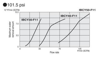
Note: The maximum amount of water removed from a volume of air in a process depends on the conditions of usage (this graph is not a guarantee). Use it as a guideline for your selection.
