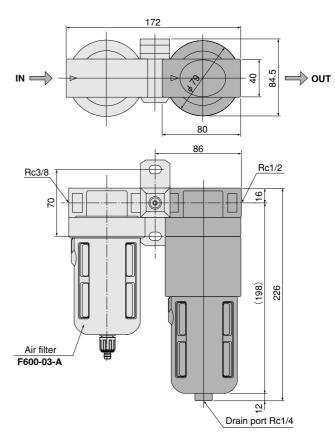
Caution: Always mount an air filter (5 $\mu$ m) in upstream of the cool separator for use.
