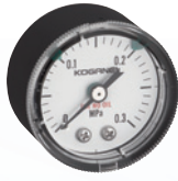
φ 40 [1.575 in] stainless steel Bourdon tube pressure gauge (0.3 MPa [44 psi] specifications)
