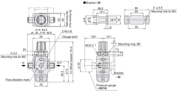
Note: The required mounting hole when the regulator is installed to a panel, etc., is  $\phi$  18.5 [0.728in.].
