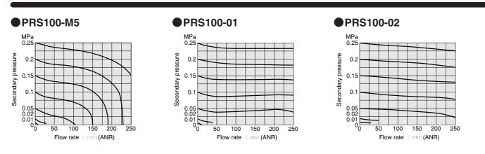
Remark: Graphs show flow rate characteristics when the primary pressure is fixed at 0.7MPa [102psi.].
