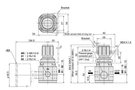
Remark: Mounting holes for the precision stainless regulator on a panel are  $\phi$ 24.5.
