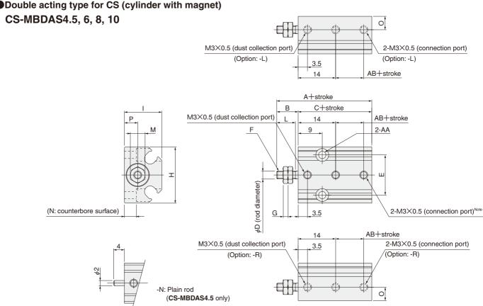
Note: When selecting the optional port location code -R or -L, the standard connection port comes with a plug.
