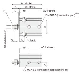
Note: When selecting the optional port location code -R or -L, the standard connection port comes with a plug.
