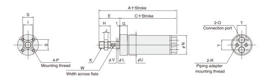
● Single foot mounting type TWDA Bore size X Stroke -HA-1A
