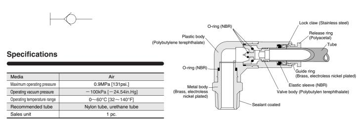
Remark: Supplied with a gasket or sealant coated.
