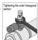
Caution: While the quick fitting sealant can be reused a number of times, the thread on the mating part may also be adhered with sealant. Always clean out the inside of the equipment's female thread.
