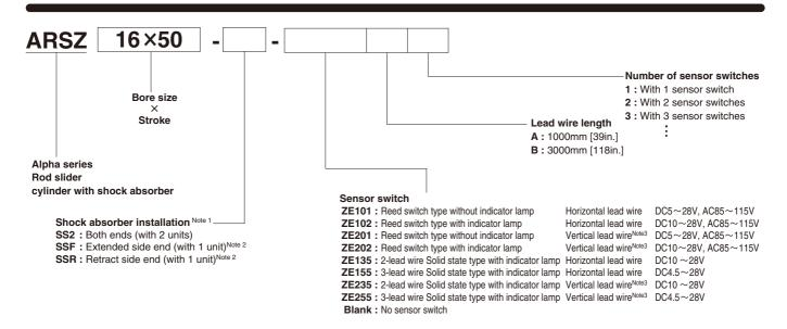
Notes: 1. A cylinder with shock absorber is not available for the end keep cylinders.
