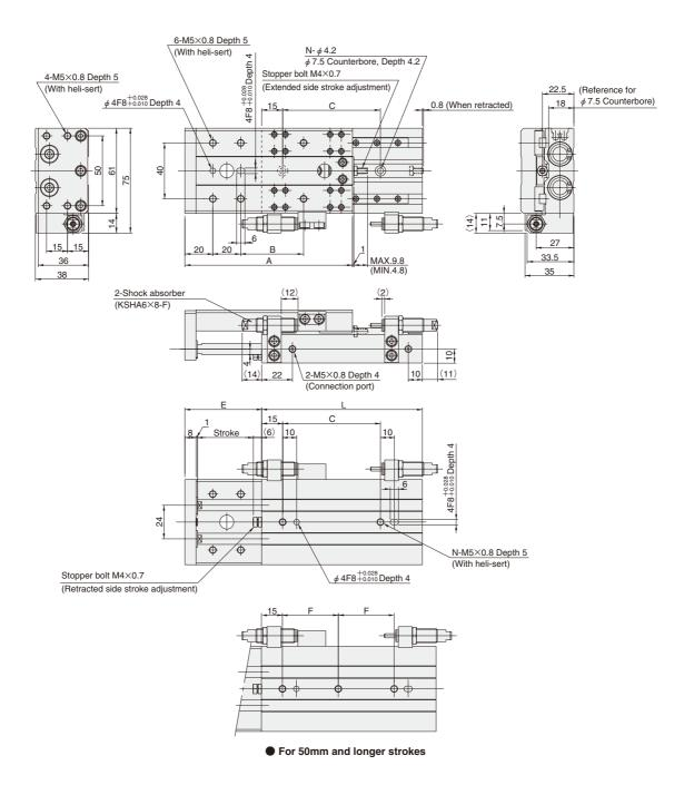
Notes: 1. The drawings above show **-SS2** with shock absorbers on both ends (with 2 units).
