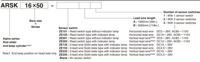
Note2: In the vertical lead wire type, the lead wire protrudes at a right angle to the sensor switch.
