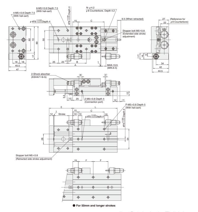
Notes: 1. The drawings above show **-SS2** with shock absorbers on both ends (with 2 units).
