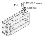
Cautions: 1. It is dangerous to release the lock when load (weight) is present on the piston rod, because it may cause the unintended piston rod's extension, etc. In this case, always supply air to the connection port opposite the one adjacent to the locking mechanism before releasing the locking mechanism.
