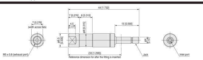
Note 1: Use the mini type quick fitting  $\phi 4$  [0.157 in] to pipe the inlet port (jack).
