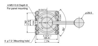
Detailed diagram for machining panel mounting holes
