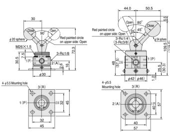
Notes: 1, Although the 125V lever is set on the 1(P) port side in the normal condition, it can be positioned in 360° range.
