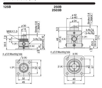
Note: For the normally open type, the exhaust port 3(R) is on the opposite side.
