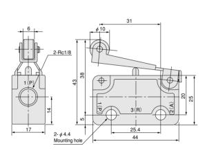
One way roller-cam type KMO-2 KMO KMO-11
