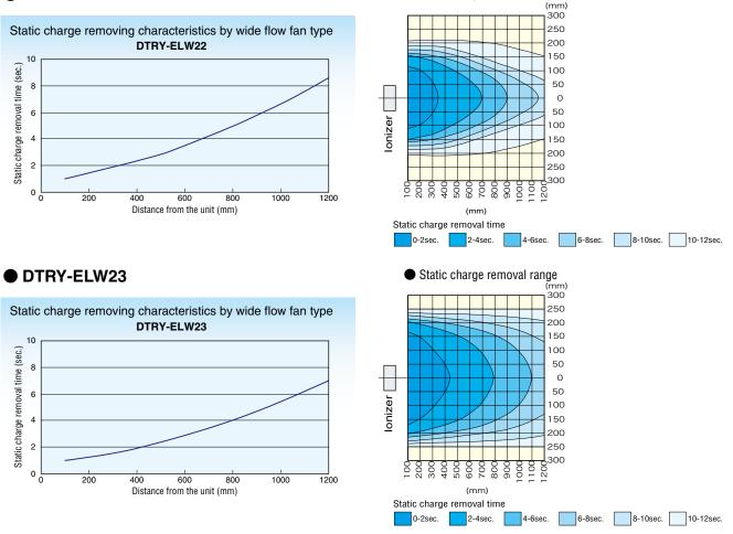
Notes: 1. The measurement method uses a 20pF and  $\Box$  150mm charged plate monitor, measured under Koganei's general measurement conditions. 2. Static removal time means decaying time from  $\pm$  100V to  $\pm$  100V, without a filter and while at the maximum air flow rate.
