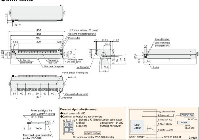
Notes 1: ON/OFF of the power to the lonizer should be done at the input side (+24 VDC side). 2: Ground for power and ground terminal are connected inside.
