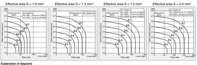
At supply pressure of 0.5 MPa, and flow rate of 49  $\ell/min$  (ANR), valve outlet pressure becomes 0.4 MPa.
