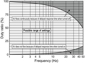
Note: The above two graphs show reference values for K2 Series types with an ON response time of 3.0 ms and an OFF response time of 10 ms.
