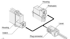
When removing the connector, make sure that the lever's claw is disengaged from the indent of the housing before pulling the connector out. Pulling out the connector while the lever's claw is still engaged will damage the housing.
