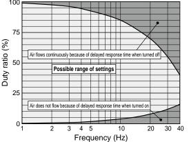
Note: The above two graphs show reference values for K3 and K4 Series types with an ON response time of 4.0 ms and an OFF response time of 15 ms.
