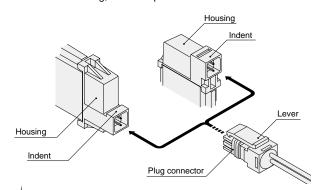
When removing the connector, make sure that the lever's claw is disengaged from the indent of the housing before pulling the connector out. Pulling out the connector while the lever's claw is still engaged will damage the housing.
