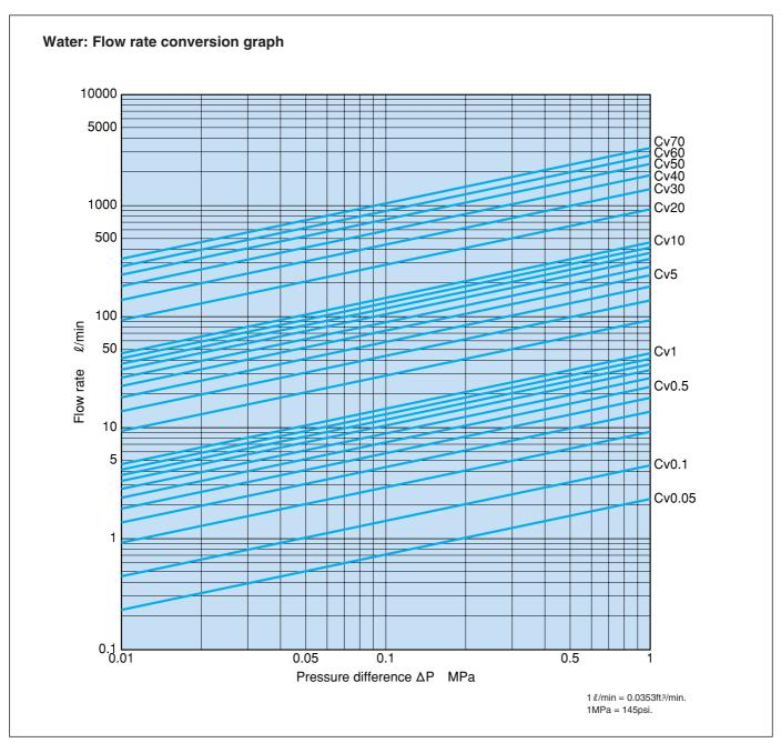
Note: The pressure difference  $\Delta P$  in the graph shows the pressure difference between the primary (upstream) gauge pressure P1 and secondary (downstream) gauge pressure P2.
