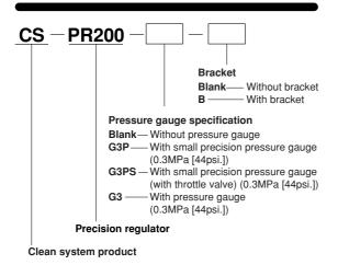
Remark: For details of the **G3** pressure gauge, see **G3-40** of the General Catalog of Air Treatment, Auxiliary, Vacuum.
