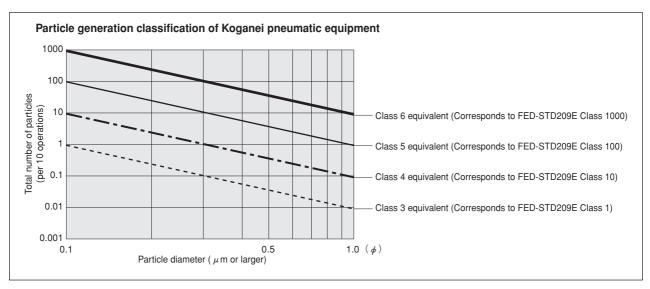
Remarks: 1. In the above table, product performance in terms of the number of particles generated per 10 operations is expressed as the upper limit of particles corresponding to the equivalent JIS or ISO class.
