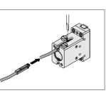
Caution: Care must be exercised that a sensor switch cannot be mounted when the body is installed by using thru holes, as shown in the diagram to the right.
