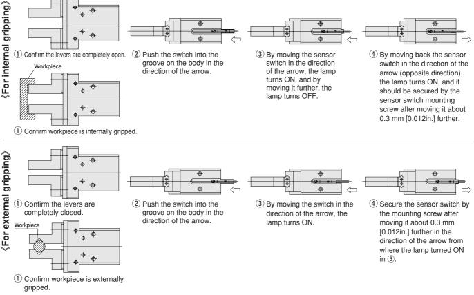
Remark: ① shows the desired location for the switch to turn ON. Install and adjust it in accordance with  $① \sim ④$  above.
