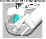
②Lift the in port in the direction of arrow 1 to remove it in the direction of arrow 2 from the semi-circle area.
