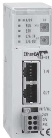
K3: EtherCAT input/output module supported
